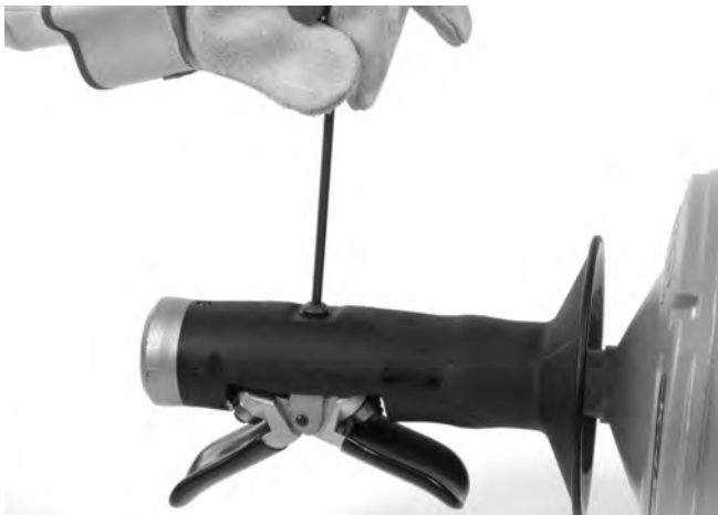
Figure 12A – Removing AUTOFEED Screw
