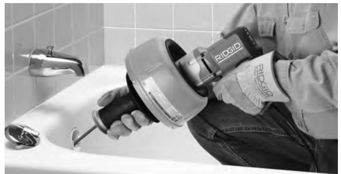
Figure 9 – Push Cable Down Drain Line
