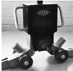
2. Tighten Long Arbor onto motor unit
