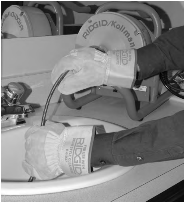
Figure 9 – Manually Feeding Cable
