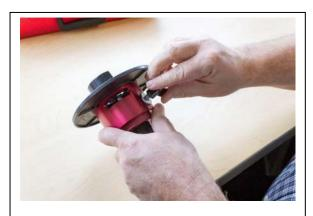
3. Replace washer. Insert adjustment knob and tighten completely.
