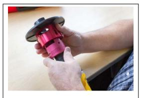
2. Slide adapter plate onto end of grinder and locate threaded hole/screw hole in the center of slot.
