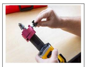
1. Unscrew black thumbscrew adjustment knob from die grinder. Remove washer.
