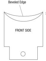
Use a high-speed dremeltype tool to flatten top edge of blade (approximately 1/32" wide flat).
